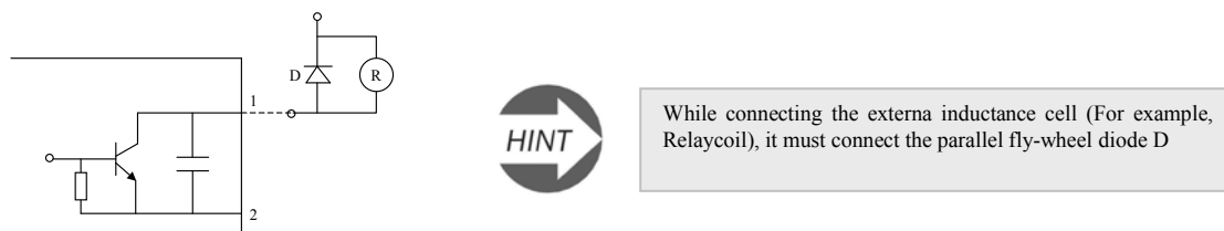
Fig.6-13 Inner wiring diagram of output terminals
