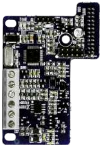
IOV-B106 used for air compressor controller to access V series / E280 series
